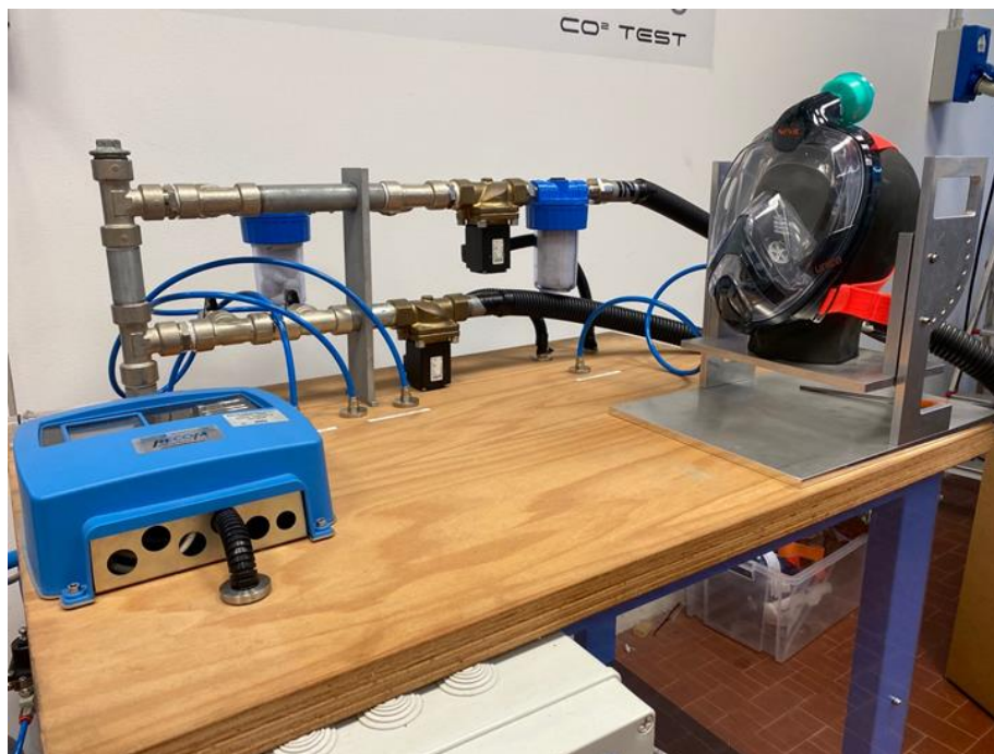
Figure 2-4: FF mask, assembled on the Sheffield head
