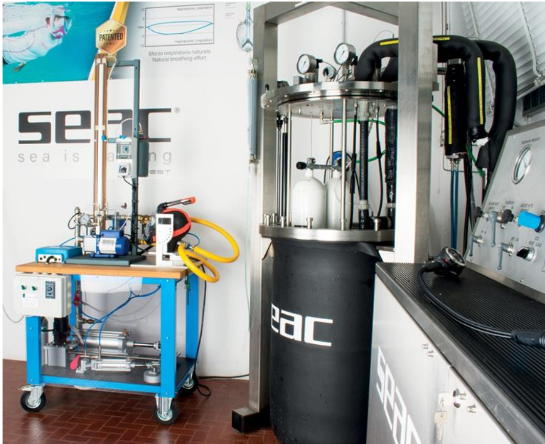
Figure 2-5: FF mask, assembled on the Sheffield head connected to the ANSTI Machine
