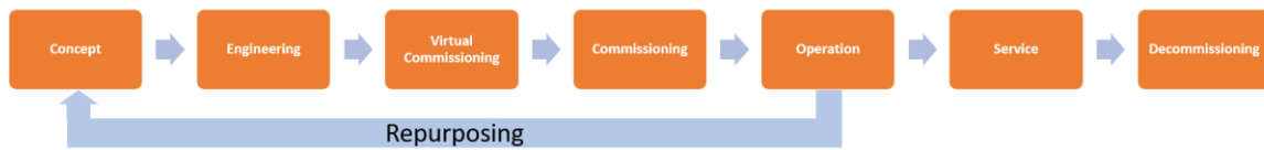
Figure 90 - Detail of the product lifecycle of a production system and the repurposing phase
